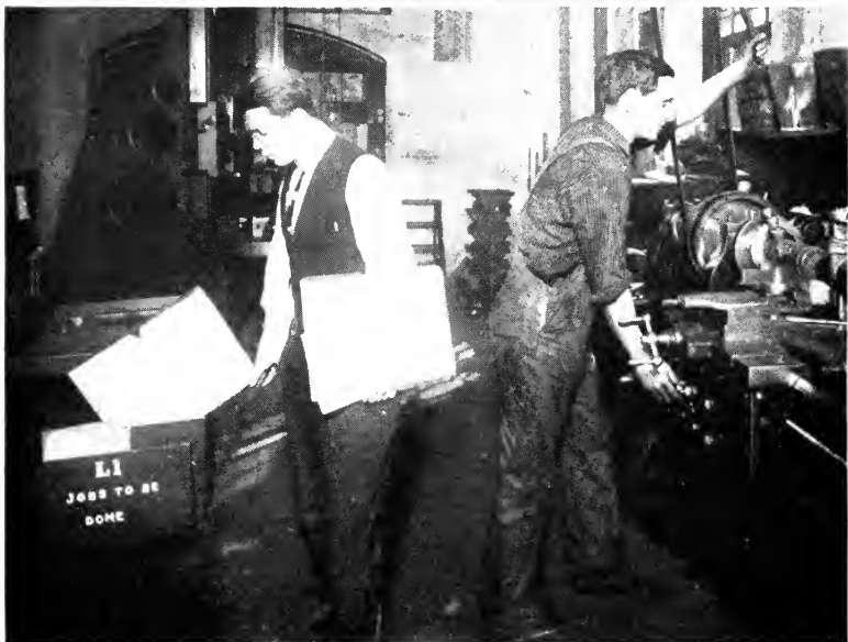
Accurate records of production must be kept at the manager's desk and at the machine. In the manager's office of a stove company (above), the supply of material is kept three weeks ahead of demand by means of the schedule shown (See Chapter V). Under scientific management, orders, drawings and instruction cards are taken to each workman before the previous job is finished
